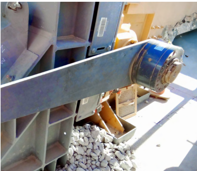
Low Speed Backstop FRHD with special torque arm
