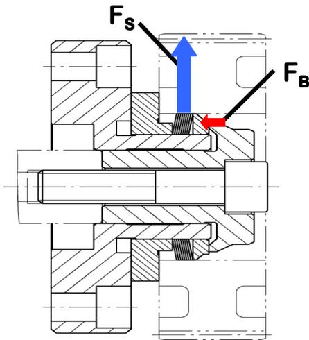
Fig. 2.1 Clamping mandrel with bonded disc pack
