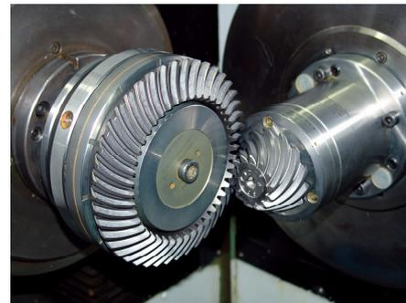
Fig. 14.2 Clamping mandrel for automotive crown gear lapping and testing
