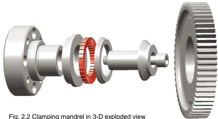
Fig. 2.2 Clamping mandrel in 3-D exploded view
