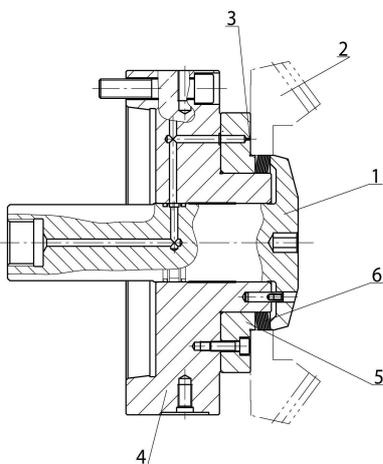
Fig. 13.1 Clamping mandrels used to mill lorry crown gears
