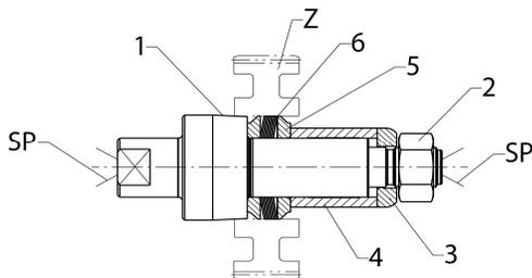
Fig. 12 Clamping mandrel for gear noise testing
