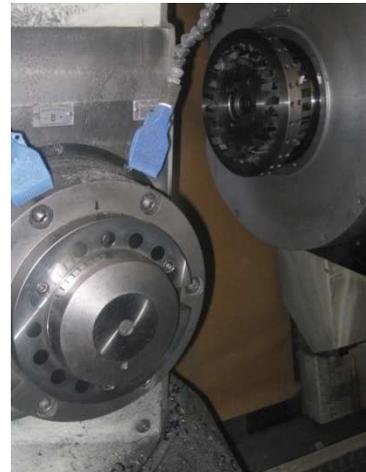
Fig. 13.2 Clamping mandrel used to mill lorry crown gears
