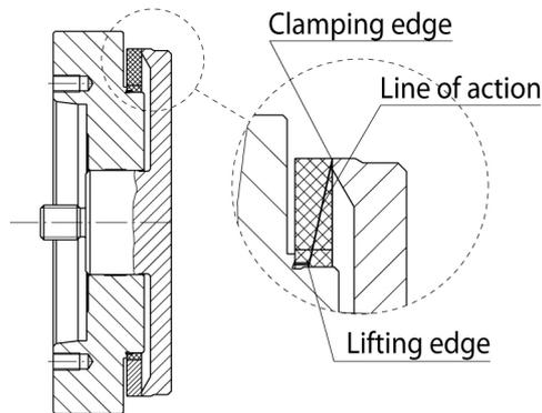
Fig. 7 disc clamping element
