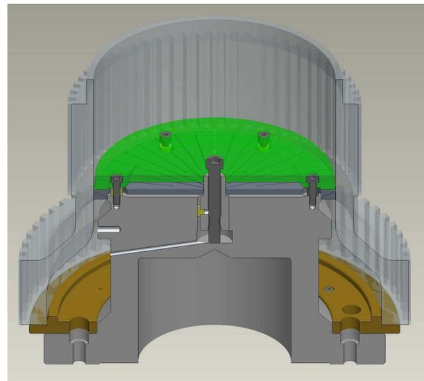
Fig. 19 Flat-mandrel for transmission bell housing – 3-D view
