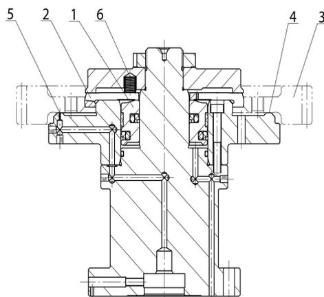
Bild 15.1 Clamping mandrel for grinding automotive spur gears
