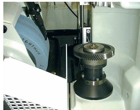
Fig. 15.2 Clamping mandrel used to grind automotive spur gears
