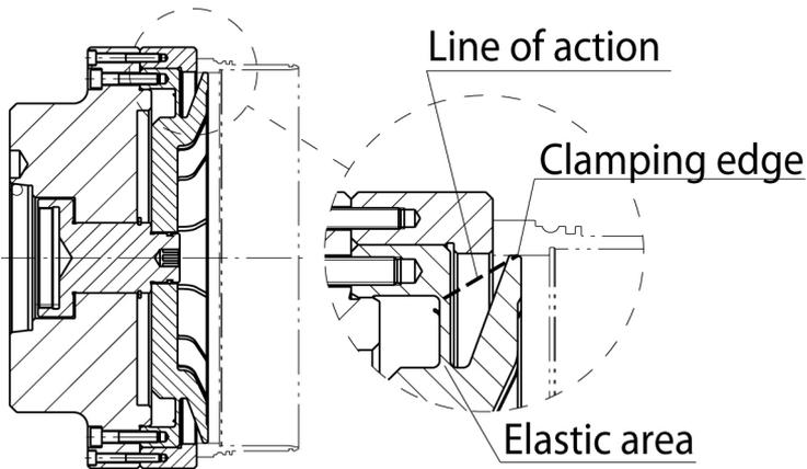
Fig. 9 Diaphragm clamping element
