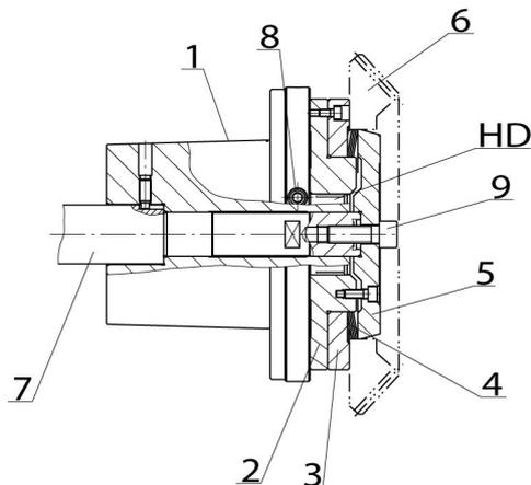
Fig. 14.1 Clamping mandrel for lapping and testing automotive spur gears
