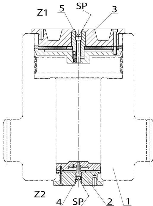
Fig. 16 Flat-mandrel clamping elements as centring inserts in a hollow shaft.
