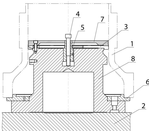
Fig. 19 Flat mandrel on machine table for transmission bell housing
